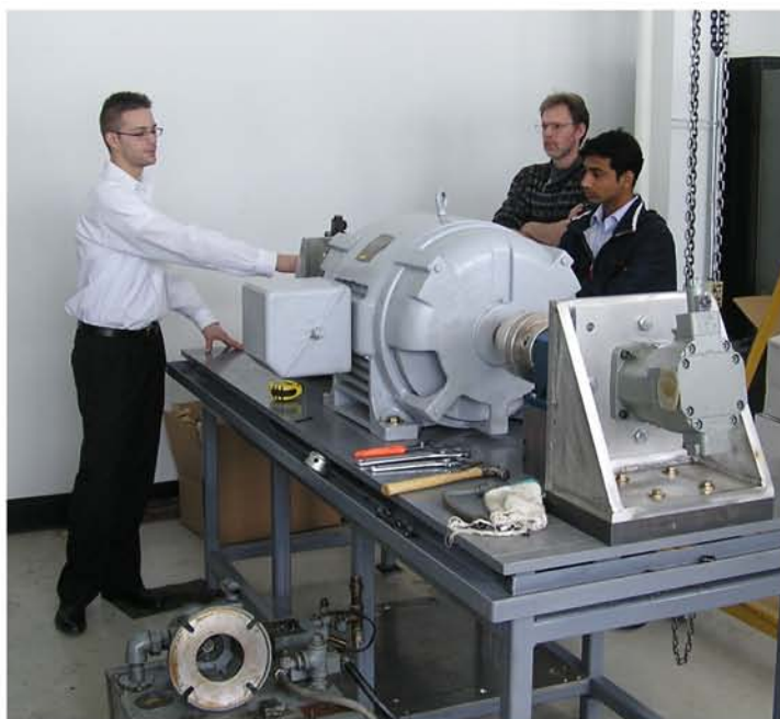
UT Mechanical Engineering masters student, Chris Schroeder explains the hydraulic hybrid pump/motor test stand to Dr. Mark Schumack, UDM, and Sujay Bodke, graduate ME student at UDM. Dr. Schumack leads the team that will create a virtual replica of the physical test stand for use in a teaching module.
